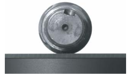
Image of a long object viewed along its field depth. The depth of field of OE telecentric lenses can hardly be achieved by other telecentric lenses.
