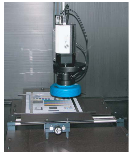
Fig. 15: a double-sided telecentric lens is interfaced with a tunable LCD filter in order to perform high resolution colour measurements. The image-side telecentricity ensures that the optical bandpass is homogeneous over the entire filter surface and delivers an even illumination of the detector, provided the object is evenly illuminated too.
