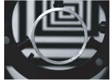
Fig. 8: Common optics showing significant image perspective error (on the left). A telecentric lens is able to cancel any perspective effect (on the right).
